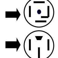
50 Amp 120/208 volt hook up \*(NEMA #14-50P) Manufactured by Hubbell, part # HBL9451c, HBL9452c
